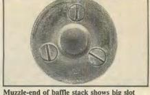
Muzzle-end of baffle stack shows big slot screw heads for easy disassembly.
